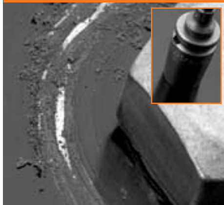
Standard socket – Heavy Damage
