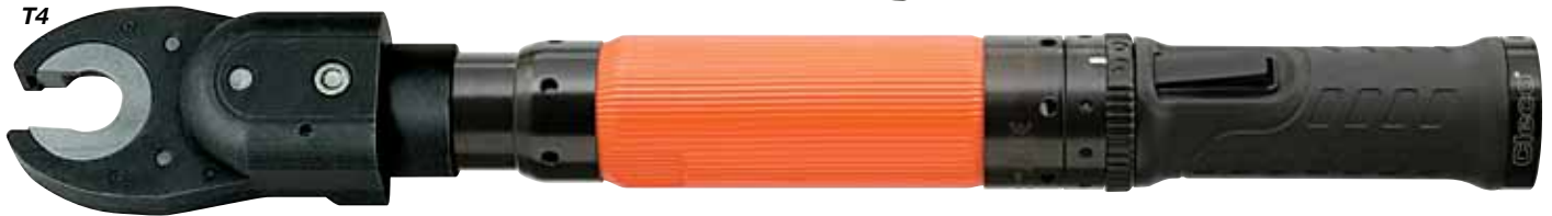
The 48ET tube nut wrench alternates the direction of rotation each time the lever is actuated. When rotating in reverse, the socket will stop at the open position.
